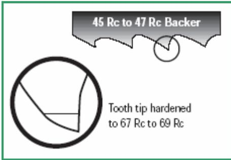
**IC Enduro** is application-designed for all bundles of solids, tube or structurals - even large cross-section structurals. It cuts faster and quieter and lasts longer - a winning combination!
