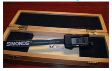
This gauge is a modified digital caliper with a magnetic back. The magnet holds the tool on the blade while it is being tensioned. The tool measures the distance the blade stretches to the nearest half thousandth of an inch, 0.0005. It works on the same principle as the precision dial indicator. It is an affordable troubleshooting tool all bandsaw operators should have and use. It comes with a user's guide and owner's manual. Battery operated.
